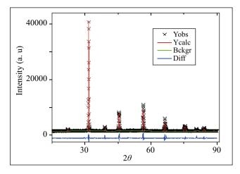
**Figure 2.** X-ray diffraction pattern for  $Sr_2SbMnO_6$  ceramics after Rietveld refinement of the crystal structure at room temperature.
