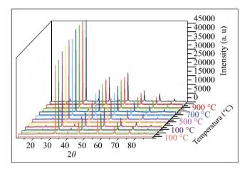
**Figure 3.** Temperature evolution of the X ray diffraction pattern of  $Sr_sSbMnO_c$ .
