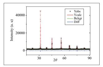
**Figure 4.** Observed, calculated and difference plots of the X-ray diffraction pattern for  $Sr_2SbMnO_6$  after Rietveld refinement at 600 °C.
