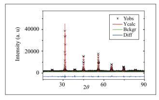
**Figure 5.** Rietveld refinement of the X ray diffraction pattern for Sr,SbMnO<sub>6</sub> ceramics at 800 °C.
