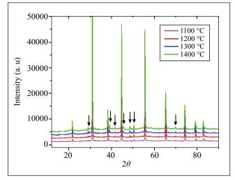
Figure 6. Diffractograms obtained for the temperature range from 1100 to 1400 °C. The arrows show the presence of other structural phases.
