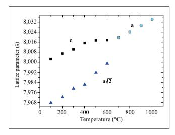
Figure 7. Temperature dependence of the lattice parameters show the continuous transition to the cubic structure above 700 °C.
